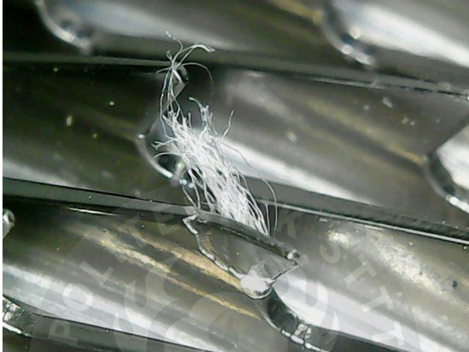
Lampiran 1.1 Wire opening roller cacat retakan
