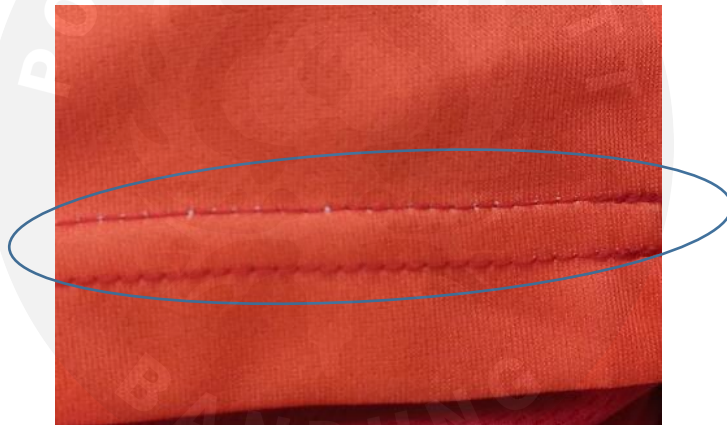
Figure 1.1 Sewing Defect on T-Shirt Style YOB 23070
